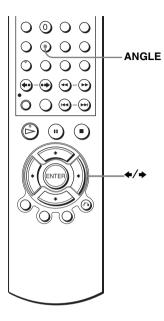
ANGLE Press ANGLE during playback. The angle number appears on the display. The number after the slash indicates the total number of angles. Press  $\star/\star$  repeatedly to select the angle number.
